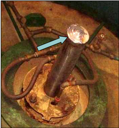
Circulating water pump with shaft break at drive keyway due to excessive design stresses (Shaft is too skinny)
