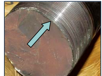
Boiler Feed Pump Shaft with Fatigue Failure in Threaded Area
