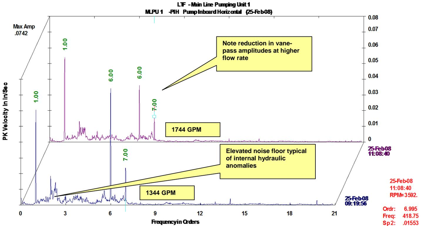
Figure 8 – PIH spectra at different flow rates exemplifying the reduction of vane-pass amplitudes at higher flow rate
