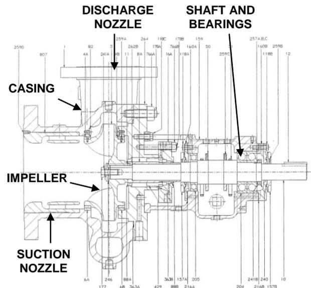
**Figure 1 – Typical Centrifugal Pump**
