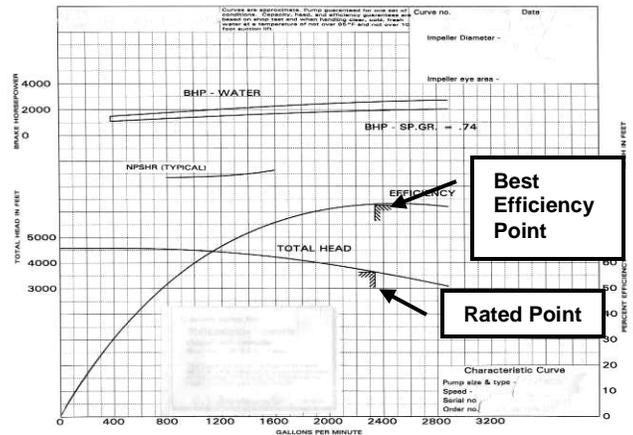
Figure 3 – Typical Pump Characteristic Curves
