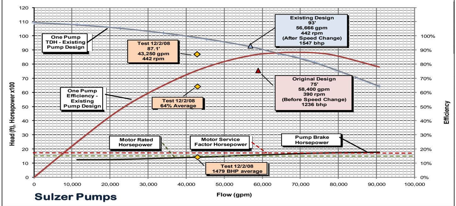
FIGURE 5: MEASURED HYDRAULIC PERFORMANCE
