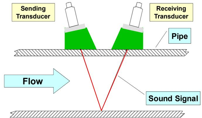
**FIGURE 4: TWO PASS ULTRASONIC FLOW MEASUREMENT THE SOUND SIGNAL CROSSES THE FLOW STREAM TWICE FOR IMPROVED ACCURACY**
