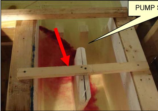
**FIGURE 8: FLOW SEPARATION**
