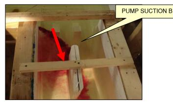
**FIGURE 8: FLOW SEPARATION**
