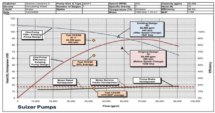
FIGURE 5: MEASURED HYDRAULIC PERFORMANCE
