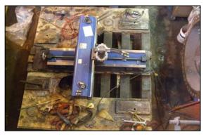
FIGURE 17: BASEPLATE AND SOLEPLATE
