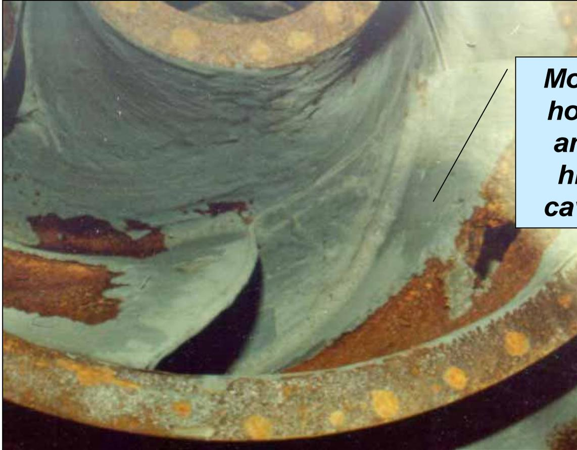
***Most coatings do not hold up on impellers and shrouds due to high velocities and cavitation/separation***
