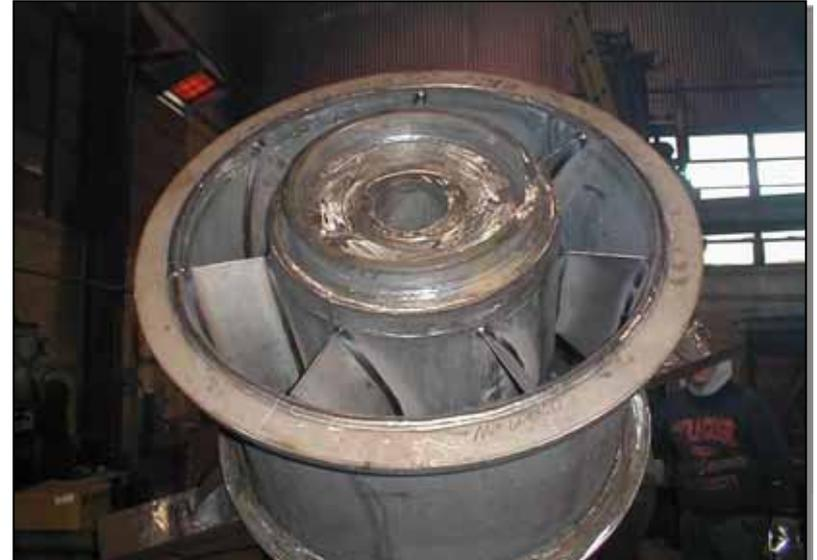
*New 316L SS Fabricated Diffusor Being Machined*
