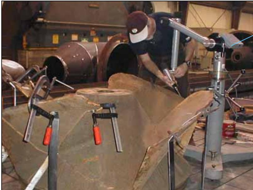
*Use the Faro Arm to obtain impeller vane geometry*
