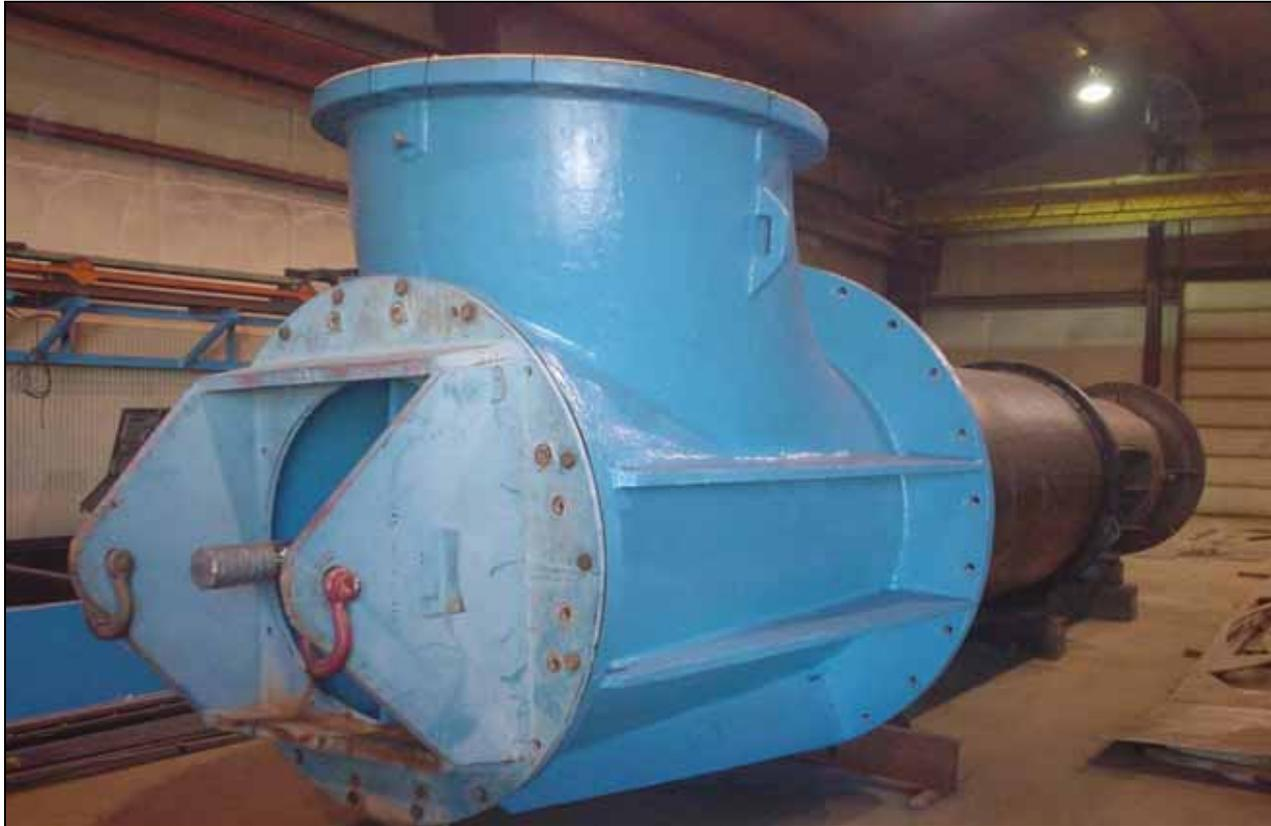
Often the Highest Design Stresses a Vertical Pump is Exposed to is During Lifting and Transportation
